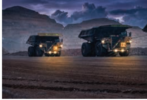
Three 36" character displays (VID-1C36-A) per haul truck. Amber LED stays legible in low light.
