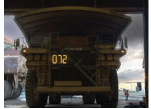
Three-digit 16" numeric display (VID-1C18-A) for unit identification. Visible up to 1,000 ft.
