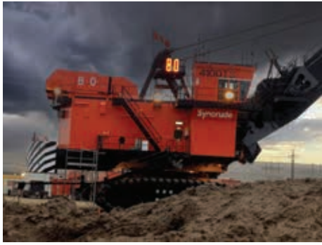
Two 36" character displays (VID-1C36-A) on an electric rope shovel. Visible up to 2,000 ft.
